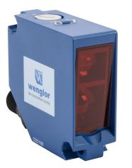
Wenglor photoelectric sensor, square, plastic, diffuse with background suppression, 0-300mm sensing distance, complementary light-on/dark-on, PNP, potentiometer, 800 Hz switching frequency, 4-pin M12 quick-disconnect.
