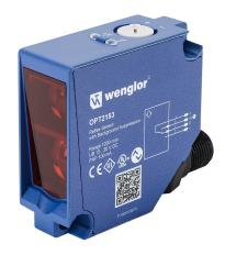
Wenglor photoelectric sensor, square, plastic, diffuse with background suppression, 0-1200mm sensing distance, complementary light-on/dark-on, PNP, potentiometer, 500 Hz switching frequency, 4-pin M12 quick-disconnect.
