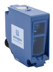
Wenglor photoelectric sensor, square, plastic, diffuse with background suppression, 50-400mm sensing distance, complementary light-on/dark-on, PNP, potentiometer, 800 Hz switching frequency, 4-pin M12 quick-disconnect.
