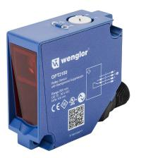
Wenglor photoelectric sensor, square, plastic, diffuse with background suppression, 0-500mm sensing distance, complementary light-on/dark-on, NPN, potentiometer, 800 Hz switching frequency, 4-pin M12 quick-disconnect.
