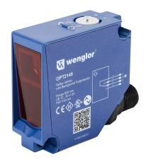
Wenglor photoelectric sensor, square, plastic, diffuse with background suppression, 0-500mm sensing distance, complementary light-on/dark-on, PNP, potentiometer, 800 Hz switching frequency, 4-pin M12 quick-disconnect.
