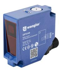
Wenglor photoelectric sensor, square, plastic, diffuse with background suppression, 0-200mm sensing distance, complementary light-on/dark-on, NPN, potentiometer, 800 Hz switching frequency, 4-pin M12 quick-disconnect.
