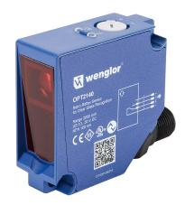
Wenglor photoelectric sensor, square, retroreflective, visible red, 0-2.6m sensing distance, complementary light-on/dark-on, NPN, potentiometer, 4-wire, 4-pin M12 quick-disconnect.
