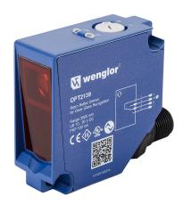
Wenglor photoelectric sensor, square, retroreflective, visible red light emission, 0-2.6m sensing distance, complementary light-on/dark-on, PNP, potentiometer, 4-wire, 4-pin M12 quick-disconnect.
