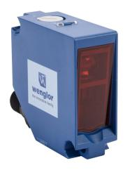
Wenglor photoelectric sensor, square, retroreflective, Class 1 red laser, 0-9.5m sensing distance, complementary light-on/dark-on, PNP, potentiometer, 4-pin M12 quick-disconnect.
