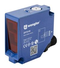
Wenglor photoelectric sensor, square, retroreflective, visible red, 0-11m sensing distance, complementary light-on/dark-on, NPN, potentiometer, 4-wire, 4-pin M12 quick-disconnect.
