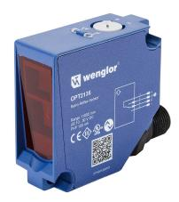
Wenglor photoelectric sensor, square, retroreflective, visible red light emission, 0-11m sensing distance, complementary light-on/dark-on, PNP, potentiometer, 4-wire, 4-pin M12 quick-disconnect.
