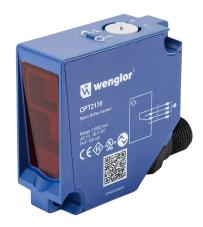
Wenglor photoelectric sensor, square, retroreflective, visible red, 0-11m sensing distance, complementary light-on/dark-on, PNP, potentiometer, 4-wire, 4-pin M12 quick-disconnect.
