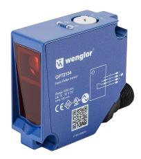
Wenglor photoelectric sensor, square, retroreflective, visible red, 0-7m sensing distance, complementary light-on/dark-on, NPN, potentiometer, 4-wire, 4-pin M12 quick-disconnect.
