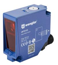
Wenglor photoelectric sensor, square, retroreflective, visible red, 0-7m sensing distance, complementary light-on/dark-on, PNP, potentiometer, 4-wire, 4-pin M12 quick-disconnect.
