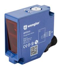
Wenglor photoelectric sensor, square, plastic housing, throughbeam receiver, 0-20m sensing distance, 10-30 VDC operating voltage, complementary light-on/dark-on, NPN, 4-wire, 4-pin M12 quick-disconnect.
