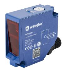
Wenglor photoelectric sensor, square, plastic housing, throughbeam receiver, 0-20m sensing distance, 10-30 VDC operating voltage, complementary light-on/dark-on, PNP, 4-wire, 4-pin M12 quick-disconnect.
