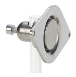
Wenglor mounting bracket, right-angle swivel, 360 degree vertical and horizontal adjustment, 304 stainless steel, 12mm rod mount. For use with OPT2012 - OPT2015 photoelectric sensors.
