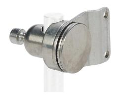
Wenglor mounting bracket, right-angle swivel, 360 degree vertical and horizontal adjustment, 304 stainless steel, 12mm rod mount. For use with OPT2024 & OPT2025 photoelectric sensors.
