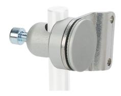
Wenglor mounting bracket, right-angle swivel, 360 degree vertical and horizontal adjustment, aluminum, 12mm rod mount. For use with OPT2024 & OPT2025 photoelectric sensors.
