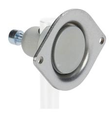
Wenglor mounting bracket, right-angle swivel, 360 degree vertical and horizontal adjustment, aluminum, 12mm rod mount. For use with OPT series 50x50mm photoelectric sensors.
