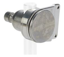
Wenglor mounting bracket, right-angle swivel, 360 degree vertical and horizontal adjustment, 304 stainless steel, 12mm rod mount. For use with OPT series 32x12mm photoelectric sensors.
