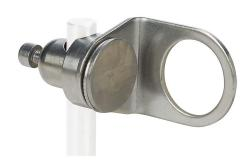
Wenglor mounting bracket, right-angle swivel, 360 degree vertical and horizontal adjustment, 304 stainless steel, 12mm rod mount. For use with 30mm sensors.
