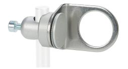
Wenglor mounting bracket, right-angle swivel, 360 degree vertical and horizontal adjustment, aluminum, 12mm rod mount. For use with 30mm sensors.
