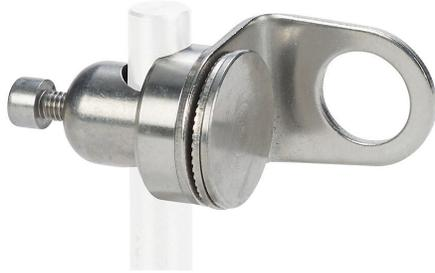
Wenglor mounting bracket, right-angle swivel, 360 degree vertical and horizontal adjustment, 304 stainless steel, 12mm rod mount. For use with 18mm sensors.
