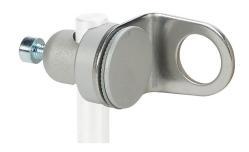
Wenglor mounting bracket, right-angle swivel, 360 degree vertical and horizontal adjustment, aluminum, 12mm rod mount. For use with 18mm sensors.
