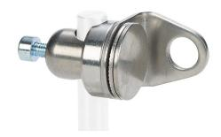
Wenglor mounting bracket, right-angle swivel, 360 degree vertical and horizontal adjustment, 304 stainless steel, 12mm rod mount. For use with 12mm sensors.
