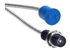
Wenglor optical fiber, glass, diffuse, statistic mixture, M18 head, aluminum, nickel plated brass jacket, 18mm sensing distance, 1m length.
