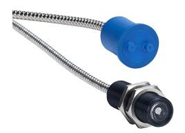
Wenglor optical fiber, glass, diffuse, statistic mixture, M18 head, aluminum, nickel plated brass jacket, 18mm sensing distance, 1m length.
