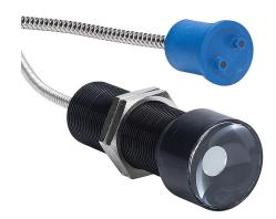
Wenglor optical fiber, glass, diffuse, statistic mixture, M30 head, aluminum, nickel plated brass jacket, 100mm sensing distance, 1m length.
