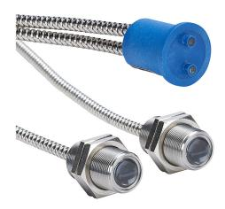
Wenglor optical fiber, glass, through-beam, statistic mixture, M18 head, aluminum, nickel plated brass jacket, 600mm sensing distance, 1m length.
