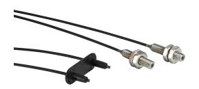
Wenglor optical fiber, plastic, cuttable, through-beam, parallel fibers, M3 head, stainless steel, polyethylene jacket, 160mm sensing distance, 2m length. Package of 2.
