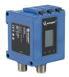
Wenglor fiber amplifier, rectangular, 3-channel, pushbutton user interface with display, NPN/PNP, programmable switching, impulse, time delay or measurement outputs, 18-30 VDC operating voltage, 4-pin and (2) 8-pin M12 quick-disconnect.
