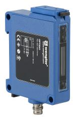
Wenglor fiber amplifier, rectangular, 1-channel, pushbutton user interface with display, NPN/PNP, programmable switching, impulse, time delay or measurement outputs, 18-30 VDC operating voltage, 4-pin M8 quick-disconnect.
