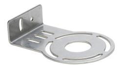
Wenglor mounting bracket, right-angle, vertical and horizontal adjustment, 304 stainless steel. For use with OPT series 50x50mm photoelectric sensors.
