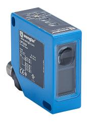
Wenglor contrast sensor, square, diffuse, white, 30-40mm sensing distance, selectable light-on/dark-on, NPN, teach-in button, 25 kHz switching frequency, plastic housing, 8-pin M12 quick-disconnect.
