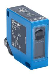
Wenglor contrast sensor, square, diffuse, white, 30-40mm sensing distance, selectable light-on/dark-on, PNP, teach-in button, 25 kHz switching frequency, plastic housing, 8-pin M12 quick-disconnect.
