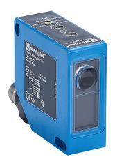
Wenglor contrast sensor, square, diffuse, white, 12-16mm sensing distance, selectable light-on/dark-on, NPN, teach-in button, 25 kHz switching frequency, plastic housing, 8-pin M12 quick-disconnect.
