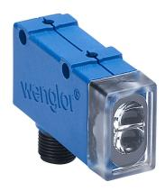
Wenglor contrast sensor, rectangular, diffuse, white, 12-18mm sensing distance, selectable light-on/dark-on, NPN, teach-in button, 5 kHz switching frequency, plastic housing, 4-pin M12 quick-disconnect.
