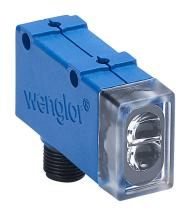
Wenglor contrast sensor, rectangular, diffuse, white light emission, 12-18mm sensing distance, selectable light-on/dark-on, NPN, teach-in button, 5 kHz switching frequency, plastic housing, 4-pin M12 quick-disconnect.
