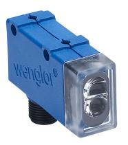
Wenglor contrast sensor, rectangular, diffuse, white, 12-18mm sensing distance, selectable light-on/dark-on, PNP, teach-in button, 5 kHz switching frequency, plastic housing, 4-pin M12 quick-disconnect.
