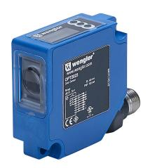
Wenglor color sensor, square, diffuse, white, 30-40mm sensing distance, selectable light-on/dark-on, NPN/PNP, teach-in button, 1.8 kHz switching frequency, plastic housing, 8-pin M12 quick-disconnect.
