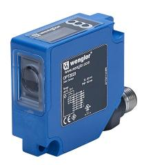
Wenglor color sensor, square, 3 color, white light emission, 30-40mm sensing distance, selectable light-on/dark-on, NPN/PNP, teach-in button, 1.8 kHz switching frequency, plastic housing, 8-pin M12 quick-disconnect.
