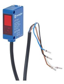
Wenglor photoelectric sensor, rectangular, polycarbonate, diffuse with background suppression, 0-1m sensing distance, complementary light-on/dark-on, PNP, teach-in button, 1 kHz switching frequency, 6.5ft/2m cable length, pigtail.
