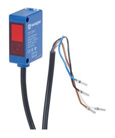
Wenglor photoelectric sensor, rectangular, polycarbonate, diffuse with background suppression, 0-1m sensing distance, complementary light-on/dark-on, PNP, teach-in button, 1 kHz switching frequency, 6.5ft/2m cable length, pigtail.
