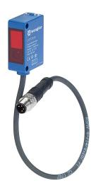
Wenglor photoelectric sensor, rectangular, polycarbonate, diffuse with background suppression, 0-1m sensing distance, complementary light-on/dark-on, PNP, teach-in button, 1 kHz switching frequency, 7.8in/200mm cable length, 4-pin M8 quick-disconnect.
