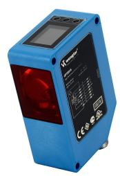
Wenglor photoelectric sensor, rectangular, retroreflective, Class 1 red laser, 0.2-100.2m sensing distance, selectable light-on/dark-on, NPN/PNP, teach-in button, 8-pin M12 quick-disconnect.
