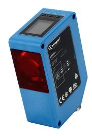
Wenglor photoelectric sensor, rectangular, diffuse, Class 2 laser light emission, 0.1-10.1m sensing distance, selectable light-on/dark-on, NPN/PNP, teach-in button, 50 Hz switching frequency, polycarbonate housing, 4-pin M12 quick-disconnect.
