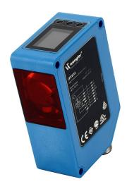
Wenglor photoelectric sensor, rectangular, diffuse, Class 2 red laser, 0.1-10.1m sensing distance, selectable light-on/dark-on, NPN/PNP, teach-in button, 50 Hz switching frequency, polycarbonate housing, 8-pin M12 quick-disconnect.
