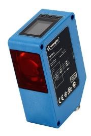
Wenglor photoelectric sensor, rectangular, diffuse, Class 1 laser light emission, 0.2-6.2m sensing distance, selectable light-on/dark-on, NPN/PNP, teach-in button, 50 Hz switching frequency, polycarbonate housing, 4-pin M12 quick-disconnect.
