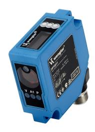
Wenglor photoelectric sensor, square, diffuse, Class 1 red laser, 0.05-3.05m sensing distance, selectable light-on/dark-on, NPN/PNP, teach-in button, 250 Hz switching frequency, polycarbonate housing, 4-pin M12 quick-disconnect.
