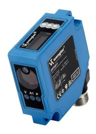
Wenglor photoelectric sensor, square, diffuse, Class 1 laser light emission, 0.05-3.05m sensing distance, selectable light-on/dark-on, NPN/PNP, teach-in button, 250 Hz switching frequency, polycarbonate housing, 4-pin M12 quick-disconnect.
