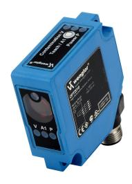
Wenglor photoelectric sensor, square, polycarbonate, diffuse with background suppression, 0-3m sensing distance, complementary light-on/dark-on, PNP, teach-in button, 1 kHz switching frequency, 5-pin M12 quick-disconnect.
