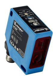
Wenglor photoelectric sensor, square, polycarbonate, diffuse with background suppression, 60-660mm sensing distance, complementary light-on/dark-on, NPN/PNP, teach-in button, 100 Hz switching frequency, 5-pin M12 quick-disconnect.
