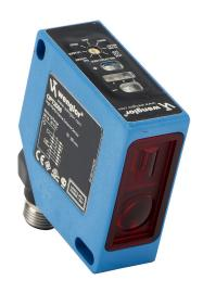
Wenglor photoelectric sensor, square, diffuse, Class 1 laser light emission, 50-350mm sensing distance, teach-in button, polycarbonate housing, 8-pin M12 quick-disconnect.
