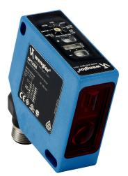
Wenglor photoelectric sensor, square, diffuse, Class 2 red laser, 50-350mm sensing distance, teach-in button, polycarbonate housing, 8-pin M12 quick-disconnect.
