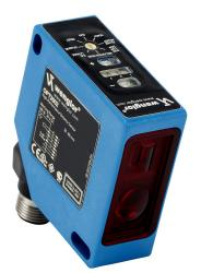
Wenglor photoelectric sensor, square, diffuse, Class 1 laser light emission, 30-80mm sensing distance, teach-in button, polycarbonate housing, 8-pin M12 quick-disconnect.
